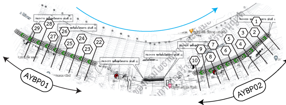
Figure 2 Plan view of the Chao Phraya Riverbank protection revetment project at Moo 10, Ban Pom Subdistrict, Phra Nakhon Si Ayutthaya District, Phra Nakhon Si Ayutthaya Province, showing site conditions, boreholes (red circles), flow direction (blue line), and electrical resistivity survey lines (diamond symbols).
